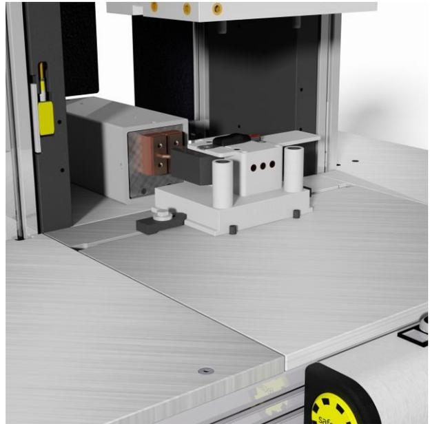
With the induction option it is possible to realize adhesion also on metallic components in one stable process step.
